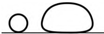
Figure 3.47 Carbon nanotubes with very large diameters flatten on a substrate, while smaller tubes largely keep their circular cross-section.
