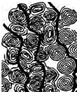
Figure 4.38 Model explaining the electrical conductivity of a carbon material consisting of carbon onions and related structures. Conductive channels develop with increasing graphitization of the material (© MRS 2002).
