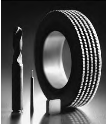
Figure 6.49 Examples of cutting and drilling tools coated with CVD diamond (© L. Schäfer).
