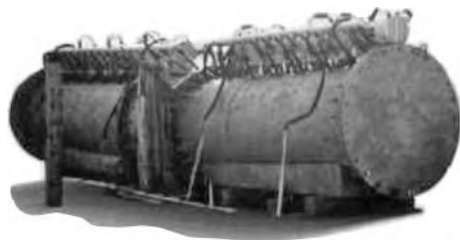
Figure 5.12 Industrial scale installation for the detonation synthesis of diamond at the Alit Corp. in Zhitomir (Ukraine). The reactor's volume is about 100\text{ m}^3 (© Alit Corp.).
