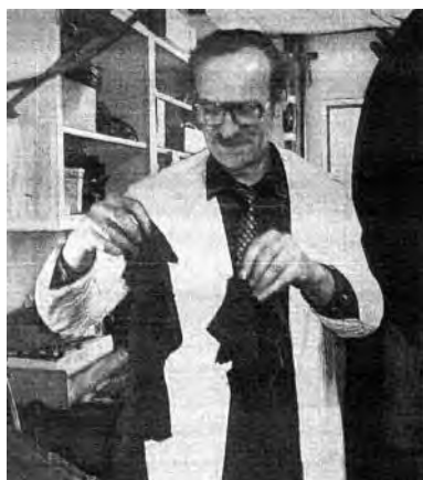
Figure 3.13 Felt-like material chiefly consisting of single-walled carbon nanotubes (© CRC Press 2005).
