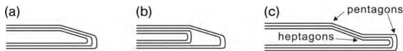
Figure 3.5 Shapes of caps on asymmetrically closed carbon nanotubes: (a) asymmetrical conical tip, (b) tip with inner cap, (c) beak-shaped tip.
